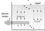
Typical convection heating applications include water and oil immersion heating, air heating, gas heating and comfort air heating.
