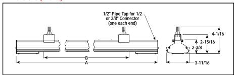
Quartz Elements are Highly Resistant to Thermal Shock but are subject to mechanical breakage. This can be minimized by careful handling and the use of protective grilles which are furnished separately.
