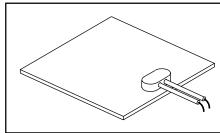
Adjustable Thermostats are available in the ranges of 50 - 300°F or 50 - 450°F. They are mounted to the heaters and covered with a durable rubber box. Adjustments can be made with either a factory provided knob or with a screw driver. Other temperature ranges available on request.
