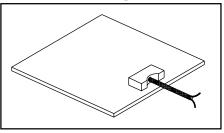
**Power Cords** can be vulcanized into the heaters either with or without plugs. Internal and external strain reliefs are used to ensure cord attachment strength and durability of the element. Ground wires, if used, can be mounted to internal grounding screens, mounting plates or foil backing. All "flying" ground wires are a minimum of 6" in length and may have a ring terminal attached for easy field grounding to your part.
