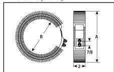
Note — Maximum temperatures are based on 25 W/ln². If elements have a lower watt density, work temperature may be increased; if watt density is higher, work temperature should be lower.
