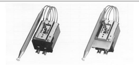
Description: PECO T125 series thermostats are single pole, single throw (SPST), open on temperature rise, snap action devices for a variety of liquid or air sensing applications. Their principal use is as a regulating control but some models may also have application as a limit control (see "Important" notice). These controls are designed for precision, durability and accuracy.
