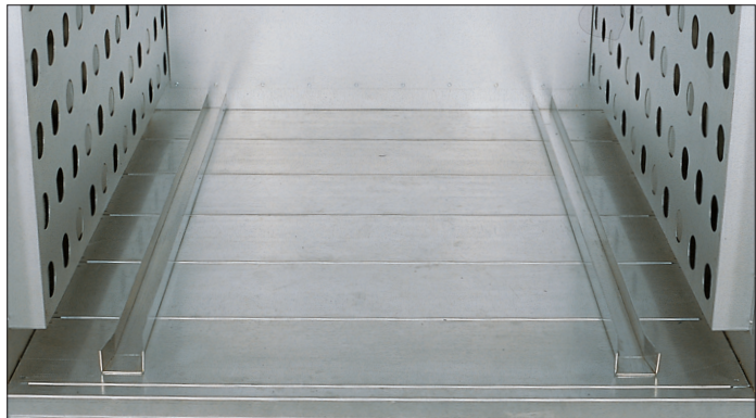
● Insulated Floor with Surface Truck Tracks used where oven will be recessed into the factory floor or loaded with an external ramp, includes drag seals on the oven doors. Total track loading limited to distributed floor loading of 100 lbs per square foot . . . . .IFSTT
