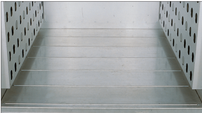
● Insulated Floor with steel plate cover , 2" for 500°F and 650°F, 3" at 800°F, minimizes heat loss and improves temperature uniformity near floor level, rated at 100 lbs per square foot distributed loading . . . . .IF
